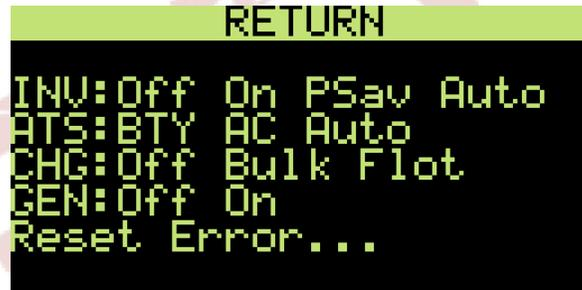
**NOTE:** Not all Commands will be visible depending on the inverter’s setup and current usage. For example, the “GEN” commands will not be visible if the Generator Start functionality is disabled.
